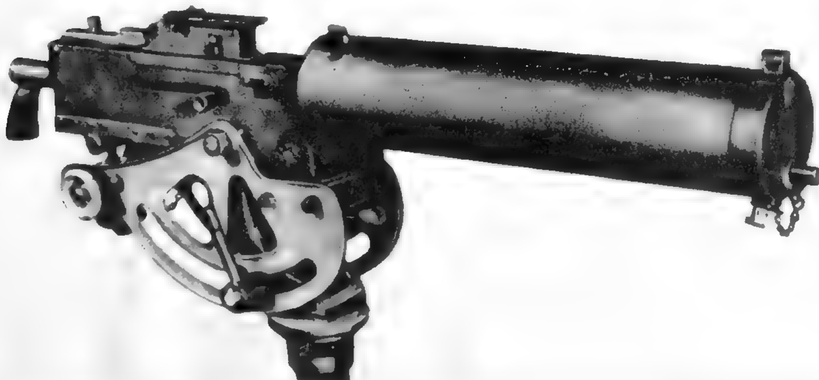
The almost elegant D7431 cradle was used with the water-cooled .30-caliber machine gun and other weapons at the outset of World War II. This cradle was developed for the tripod mount 1917A1 and was also used with the M24 mount.
